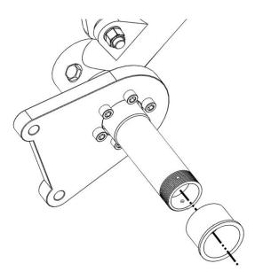
9. Drill new 0.136" diameter cotter pin holes 90° rotated from the existing holes and 1/8" outboard (toward the threaded end of the axle).
