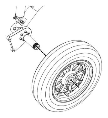
14. Install the modified axle nut.
