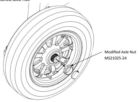
15. Tighten the nut until there is no play in the wheel bearings and then turn the nut further to the next available castellation.
