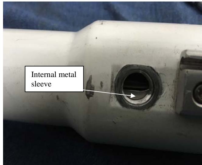
The metal sleeve shown has slid out of position.
