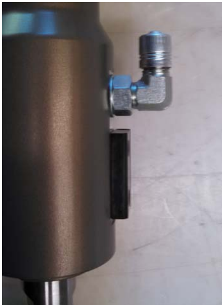
Fitting backed off 1 thread.
