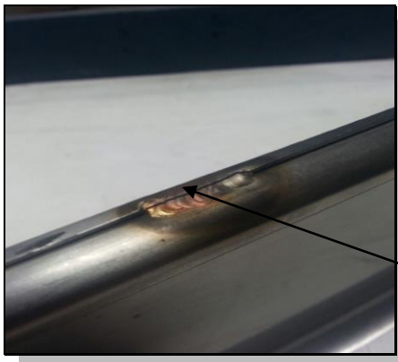
Example of Cracks in Welds
