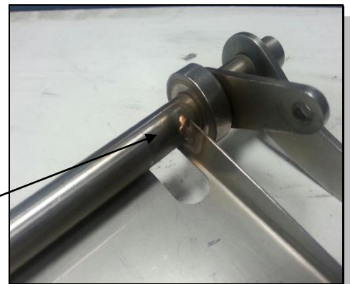
Example of Cracks in Welds
