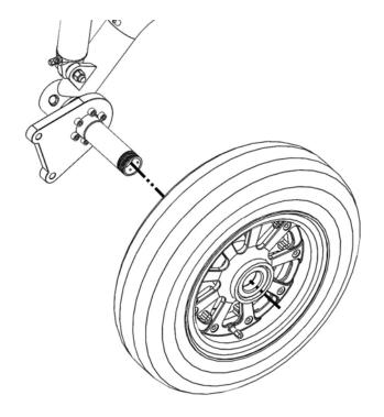
14. Install the modified axle nut.
