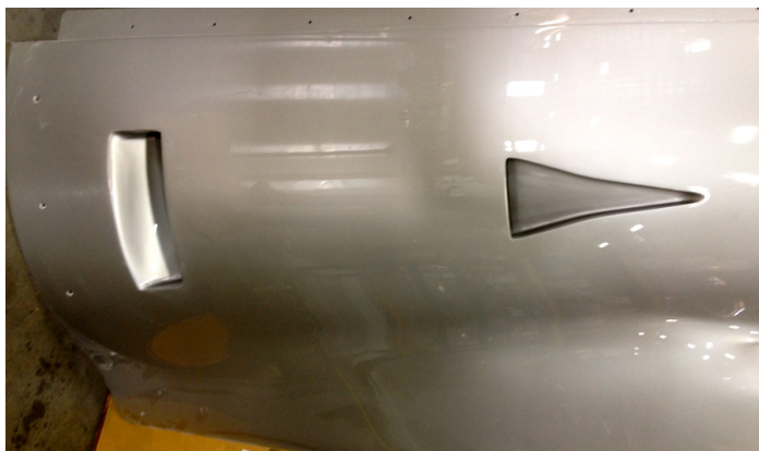
External view of intercooler installation
