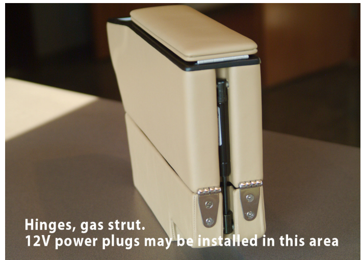
Console folded up to permit slide-over right seat access or breaker access
