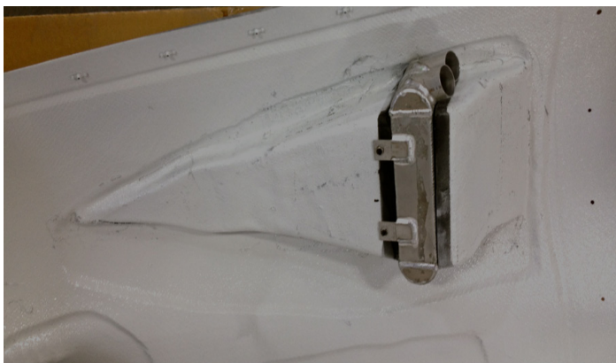
Internal view of intercooler installation
