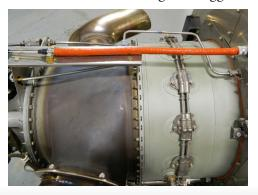
with fire-sleeve as shown in the photograph and we are amending the build manual to include this. Another vulnerable component is the
